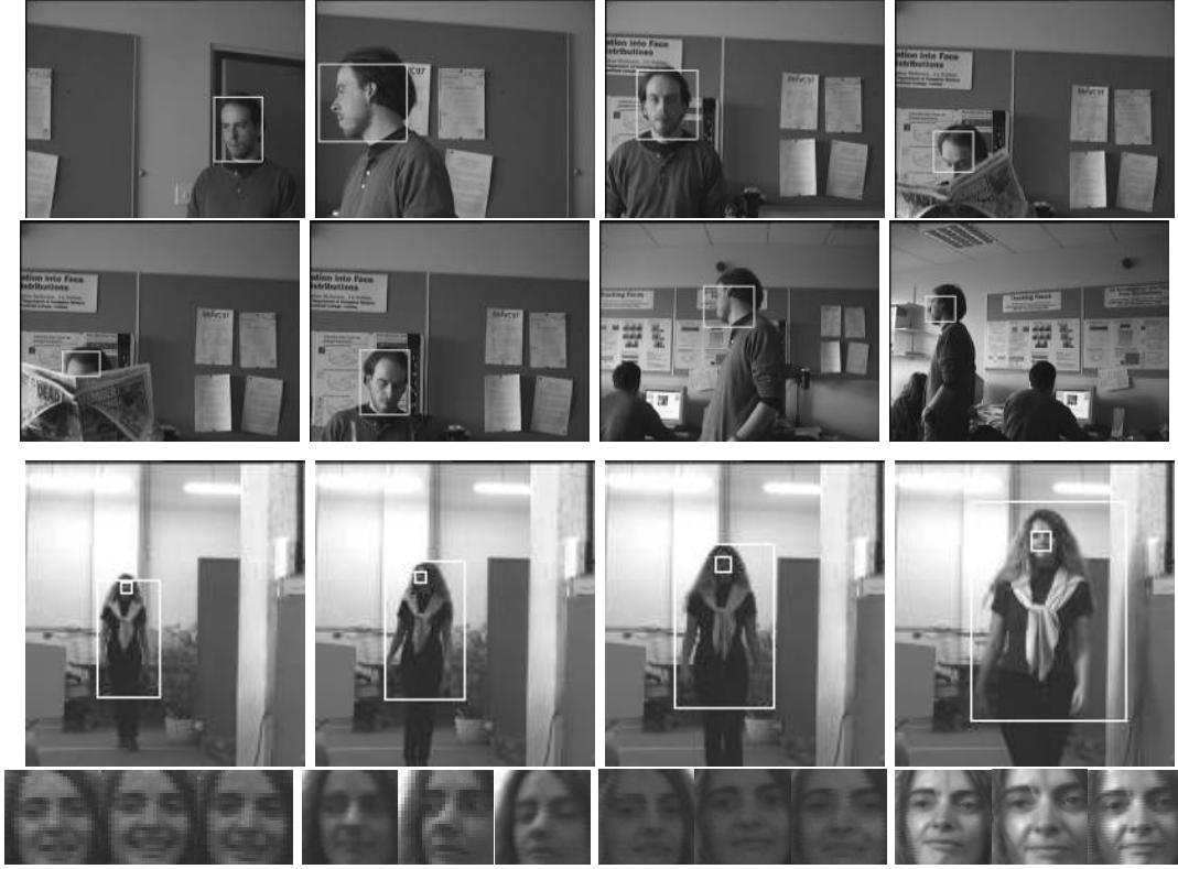
Fig. 2. Real-time tracking and normalisation in dynamic scenes using colour, motion and neural nets based face appearance models. In the first sequence the system uses a colour model to cope with large pose variations and partial occlusion whilst the camera pans and zooms. In the second sequence, approximate body bounding boxes are also shown along with aligned and scale-normalised faces.
