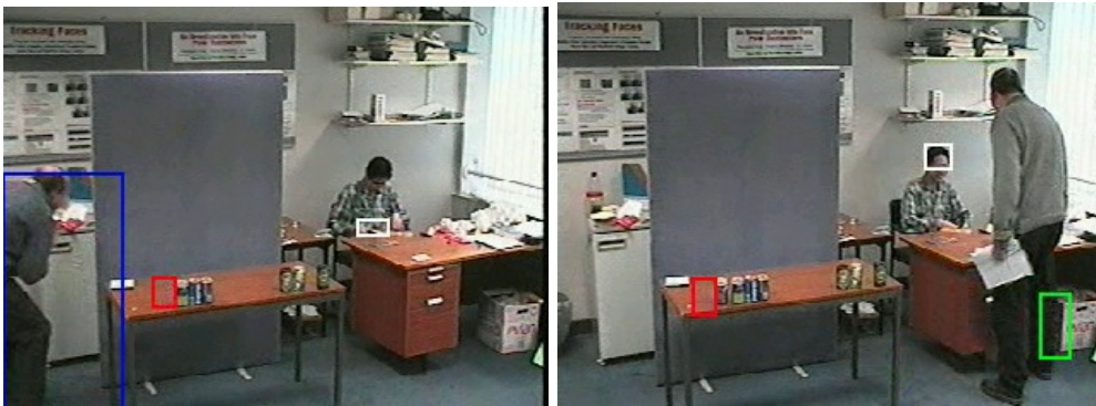
Figure 5. Clustered events using the Gaussian mixture background model to detect absolute change local events. Only the x-y positions of the events are shown.
