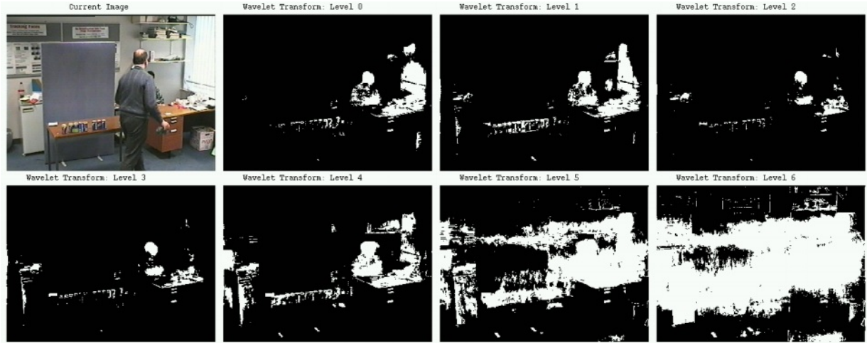
Figure 7. 7 level wavelet histogram of the shop scenario. From left to right, top to bottom, the figures are: original scene, then thresholded histograms in binary form from level 7 to level 1.
