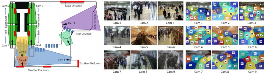
Fig. 5. The underground station layout, the camera views, and the scene decomposition results for our dataset. Entry and exit points are shown in red bars.
